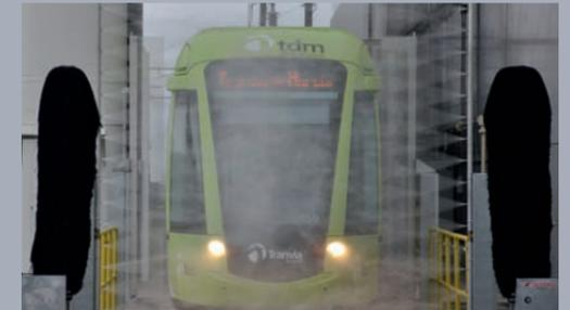
Designed to prewash the vehicles with high pressure water. The possibility to choose the water pump means the flow and pressure of the water on the vehicle can be varied by its two orientable pipes with stainless steel nozzles.
