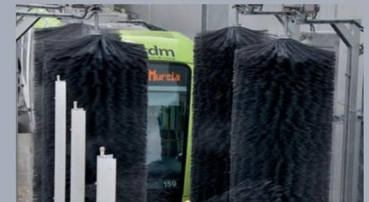
In addition to the group of four vertical brushes on the base module, 4 groups of 2 vertical brushes can be configured. These brushes are controlled by a programmable CPU, with electro-pneumatic pressure and spin force assistance sensors.
