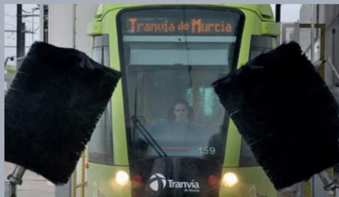
Specially designed for washing the front and rear of rolling stock with catenary. Two free standing units act as a horizontal brush with an angular positioning movement for ease of washing. Each unit has a programmable CPU, control cabinet, water circuit and centralised detergent dispensing.
