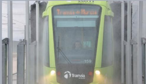
An optional extra designed to apply the chemical prewash product efficiently. Comprises two orientable pipes in stainless steel, nozzles with a non-drip system, a dispensing system, and side protectors to minimise draughts and optimise the application of the chemical product.
