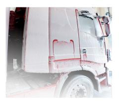
The automatic application of the chemical prewash saves time and controls consumption. Its foamy texture ensures greater efficiency in the chemical through a longer reaction time on the vehicle surface. This optional extra includes stainless steel manifolds and foamers for air mixing, a 100L pre-mix tank, and a high-pressure pump.
