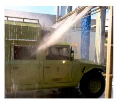
Available for the upper, lower, and top, high-pressure prewash systems are a perfect complement to the brush-wash process. These systems are recommended when washing vehicles with unique profiles. Consisting of 16-24 zero-angle nozzles (depending on the system), they use an oscillation motor (up-down) and a rotating cylinder (forward-backward) to thoroughly clean areas from different angles.
