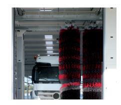
Programmable vertical side brushes clean front, back, and side surfaces while overlapping passes clean the front and rear. A variable frequency motor provides advanced mirror protection for forward and side mirrors.
