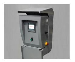
Password protected touch screen panel allows supervisors and managers to manage chemical dilution. With up to 15 wash programs in memory, managers and supervisors can select programs as weather and seasons change. This panel is required for remote program changes by ISTOBAL's support center.
